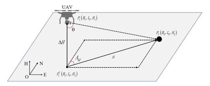
Fig. 1. Schematic diagram of the spatial geometric relationship between UAV and target object
