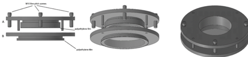
Figure 5. The figure shows a drawing of the device with the two membranes which seal the bottom of the two containers A and B and the way it is assembled.
