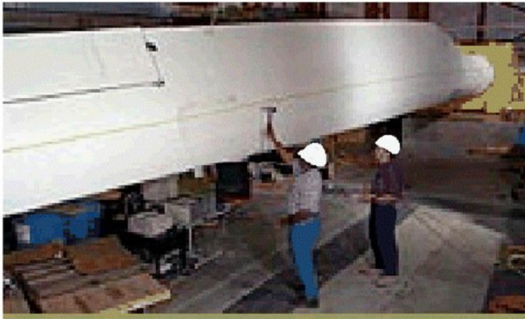
Figure 6. Wind turbine blade with a traditional trailing edge flap [23] .
