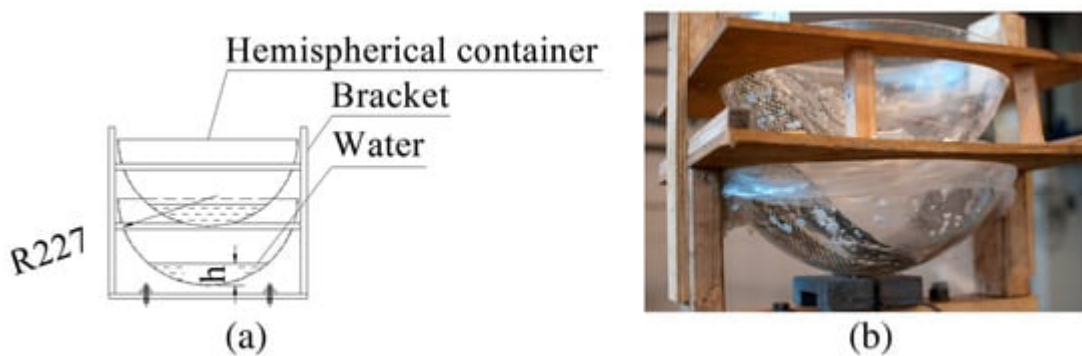
Figure 25. Spherical tuned mass damper in schematic view (a) and the actual system (b) [118].
