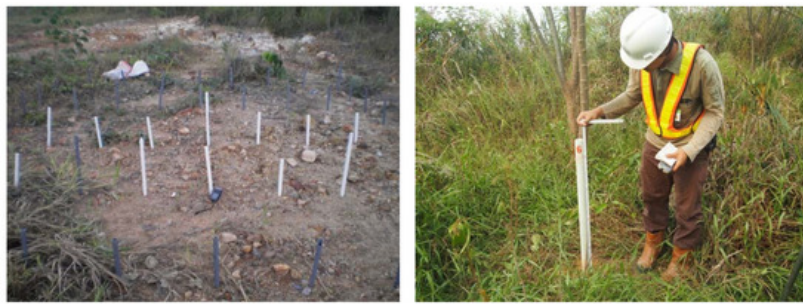
Figure 5. Measurement of the rate of erosion using erosion sticks. Photo by I. Iskandar.
