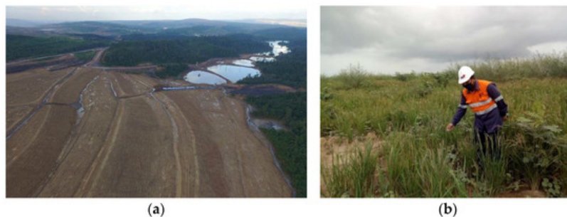
Figure 4. (a) The critical phase of the final surface against erosion and landslides after reclamation; (b) use of local upland rice and legumes as land cover crops to reduce the risk of erosion. Photo by Kaltim Prima Coal.
