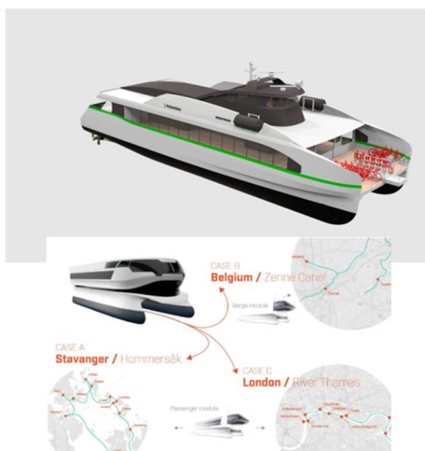
Figure 1. Image of the Stavanger Demonstrator and planned TrAM project replication studies for zero-emission, urban waterborne transport [10] https://tramproject.eu/ .
