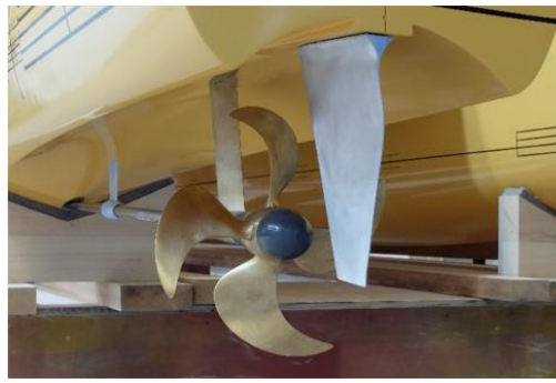
Figure 3. Close-up of the transom stern area of the tested Stavanger model, with fitted propellers, shafts, brackets and rudders [17].
