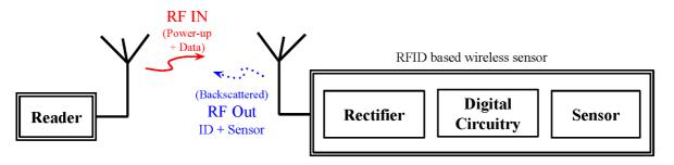
An antenna is a transducer that converts free space electromagnetic energy to guided electromagnetic energy and vice versa to enable wireless communication in an RFID system. Although any radiating structure can be termed as an antenna, the efficiency with which it can transform the electromagnetic energy plays a major role in determining its amenability for use in sensor communication [23].
