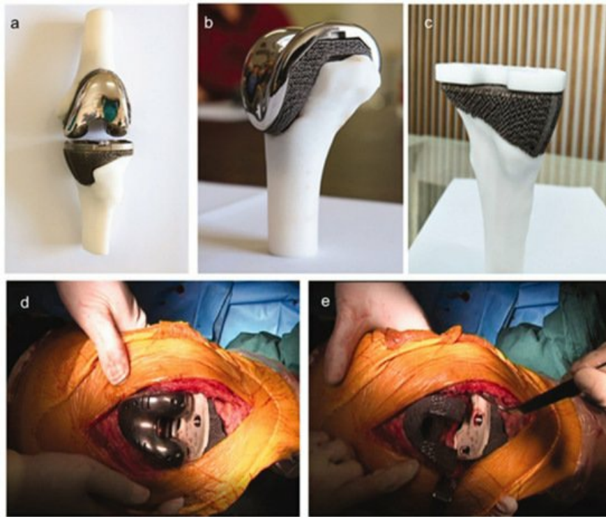
Figure 5. The printed personalized porous Ta knee prosthesis (a), distal femoral component (b) and proximal tibial component (c). The porous Ta prosthesis was inserted into distal femur and proximal tibia, respectively, during the surgery (d,e). Reprinted from ref. [159].
