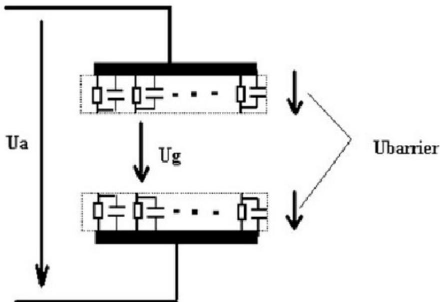
**Figure 4.** Electrical model of the RBD<sup>[24]</sup>.
