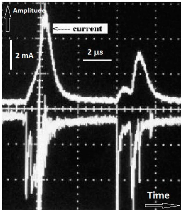
**Figure 3.** Current waveform (top curve) of a DC-powered (20 kV) RBD and discharge integrated light intensity detected by a photomultiplier tube (PMT) (curve is inverted to visually distinguish it from the current waveform). Note the correlation between the timing of the current and light pulses.
