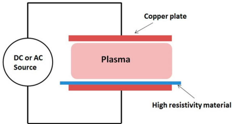
**Figure 1.** Schematic of the resistive barrier discharge.
