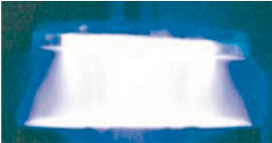
**Figure 2.** Photograph of the plasma generated by a resistive barrier discharge (RBD) in helium. The gap distance between the electrodes is 4.5 cm, and the voltage is 13 kV RMS at 60 Hz<sup>[22]</sup>. The input power is around 100 W.
