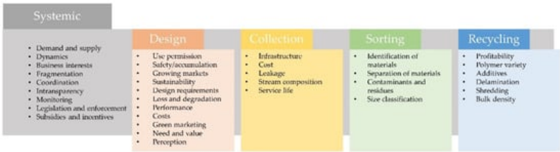
Figure 1. Hurdles to circularity of packaging focused on, but not limited to multilayer flexible packaging [7][8][9][15][16][17][18][19][20][21][22][23][24][25][26][27][28][29][30][31][32][33][34][35][36][37][38][39][40][41][42][43][44][45][46][47][48][49][50][51][52][53][54][55][56][57][58][59][60][61][62].
