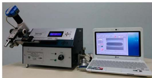
Figure 10. Oscillating spinning drop interfacial rheometer recent version.
