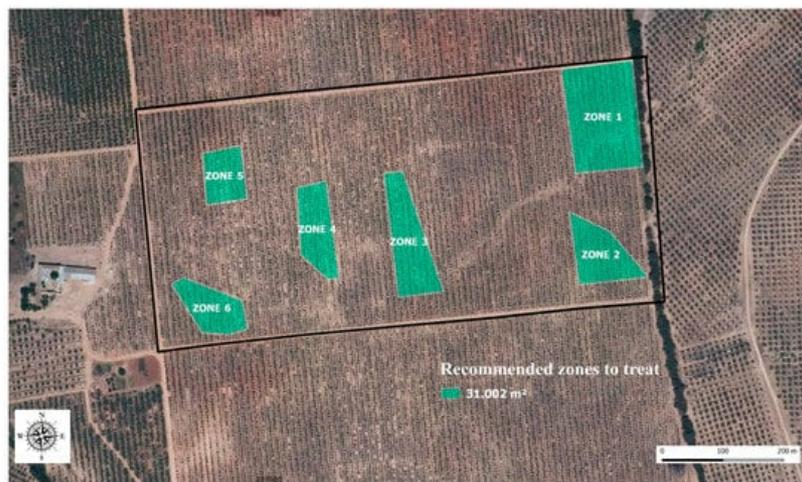
**Figure 6.** A set of field zones recommended for treatment based on the vegetation indices (VIs) maps, generated using a parrot sequoia and Yuneec CGOET mounted on a Yuneec Typhoon H hexacopter RPA for olive crops (image facilitated by MCBiodrone).
