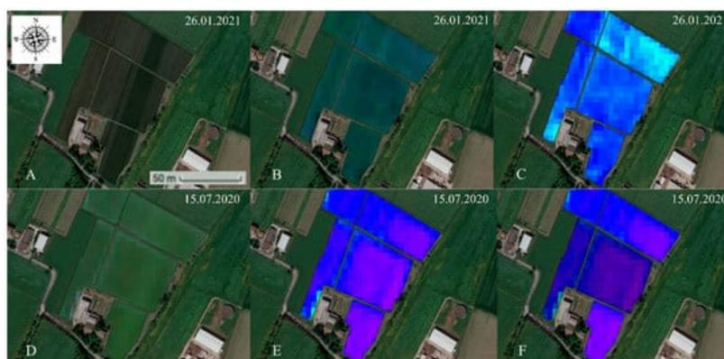
**Figure 3.** Sentinel-2 images accessed through Google Earth Engine (GEE). (A) Area of interest, (B) RGB field composition, (C) NDVI raster tile, (D) RGB field composition, (E) NDVI raster tile, (F) NDVI vector tile (Images facilitated by Graniot).
