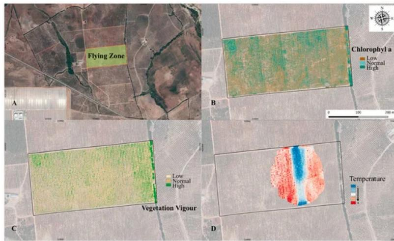
**Figure 5.** Vegetation index (VIs) maps generated through Parrot Sequoia (a multispectral camera) and Yuneec CGOET (a thermal sensor) mounted on Yuneec Typhoon H hexacopter RPA. (A) Crop area studied. (B) Map of “chlorophyll a” content based on NDRE. (C) Map for vegetation status generated based on NDVI. (D) Thermal map established using Yuneec CGOET. (Images facilitated by MCBiodrone).
