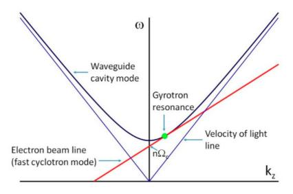
Figure 1. Gyrotron interaction illustrated by the Brillouine diagram.
