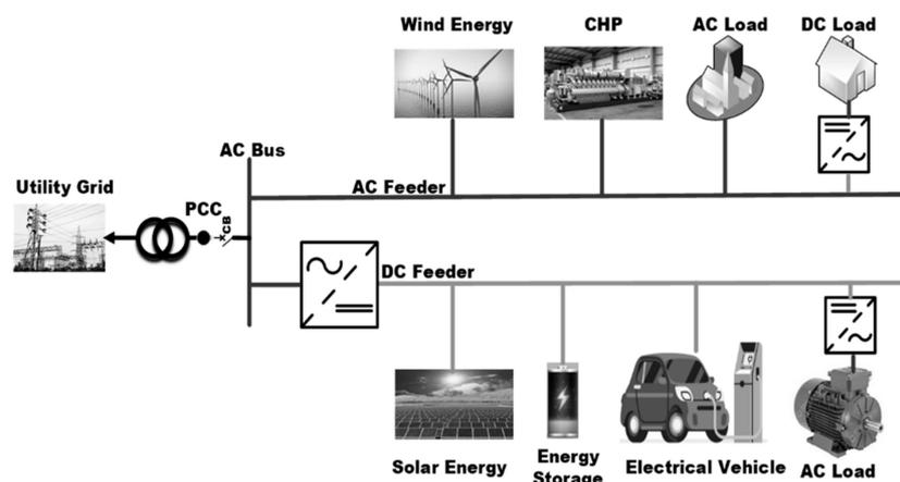
**Figure 3.** A hybrid microgrid (AC and DC systems).
