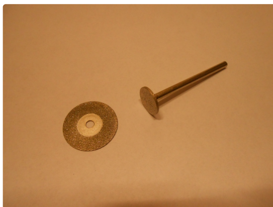
Fig. 2 - Detail of the diamond tips used for cutting and polishing the surface of clinoptilolite slabs.
