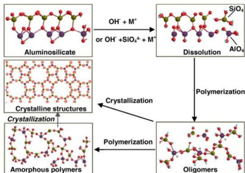
**Figure 3.** Zhang model of the geopolymerization process. Reprinted with permission from ref. [21]. Copyright 2016 Elsevier.
