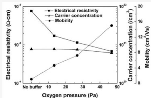
Fig. 4. Variation of the carrier concentration, Hall mobility, and resistivity as a function of the oxygen pressure of the SiO<sub>x</sub> buffer layer for GZO films deposited at room temperature. All of the GZO films were grown by a PLD method at room temperature under an oxygen pressure of 4 Pa.
