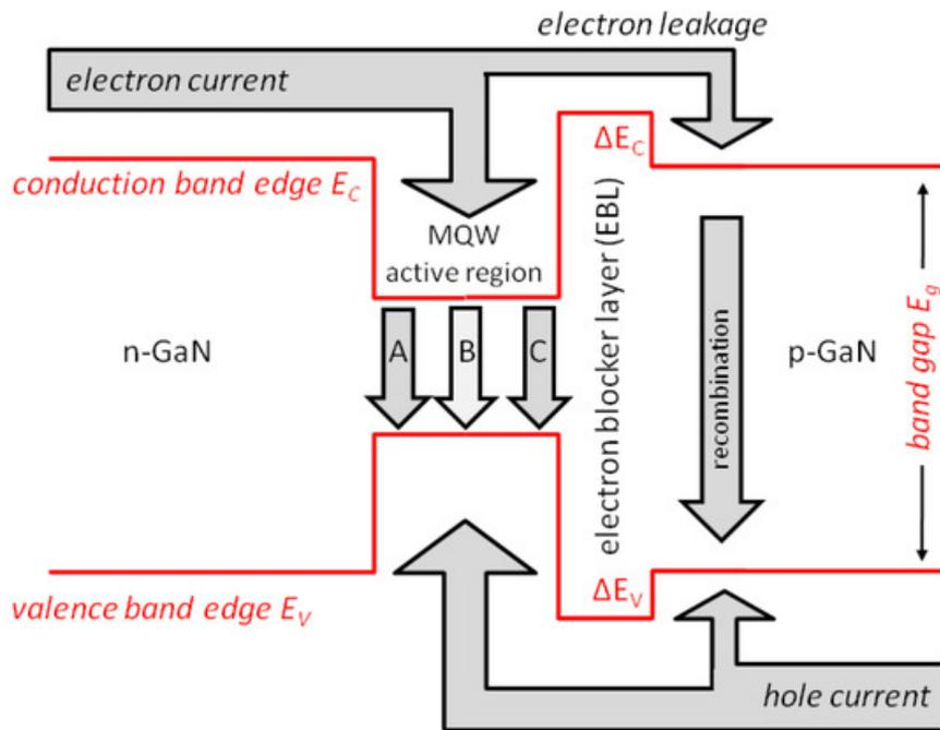
**Figure 2.** Illustration of the vertical LED energy band diagram including current flow and electron–hole recombination processes (A—defect-related recombination, B—photon emission, C—Auger recombination). Multiple quantum well (MQW) active regions typically consist of InGaN wells and GaN barriers. The electron blocker layer (EBL) is typically made of AlGaIn.
