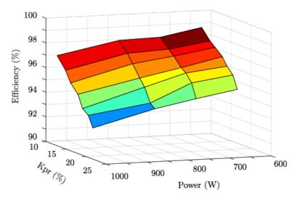
When the converter is operating below a partiality factor  $K_{pr} = 25\%$  of the total power, the dc-stage efficiency varies between 90% - 99%, as depicted in the figure. It highlight the benefit using PPCs and the relation between the partiality ratio and the efficiency.
