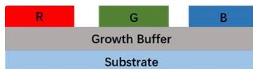
Figure 16. Multicolor LED structure with a growth buffer layer.
