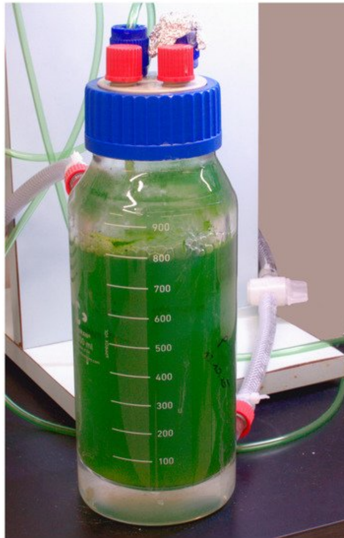
Figure 3. Culture of Arthrospira platensis in a bubble column type bioreactor. Slight foam formation and cell growth on the vessel walls were experienced (photo: M. Murkovic).
