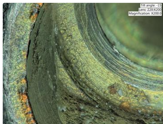
Figure 9. Closer view of an explanted implant with a hexagonal connection. Corrosion, delamination, and abrasions of the connection surface can be appreciated.
