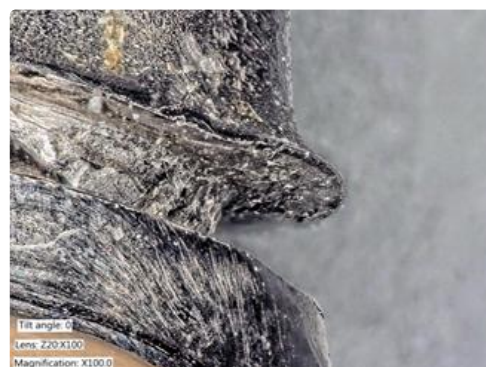
Figure 11. The evaluation of the removed crown abutment, also showed titanium particles and titanium delamination. Surface changes were also evident at the transmucosal portion of the abutment.
