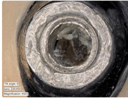
Figure 13. Evaluation of the basal aspect of the implant crown, showing deformation of the hexagon, and particle delamination.
