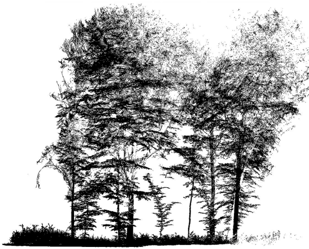
Figure 2. One of the point clouds extracted from the point cloud shown in Figure 1 using GNSS time-based point clustering. The point cloud consists of the highest number of points. The histogram of GNSS time for the point cloud is shown in the right part of the figure. The part of the histogram that corresponds to the displayed point cloud is highlighted in green.
