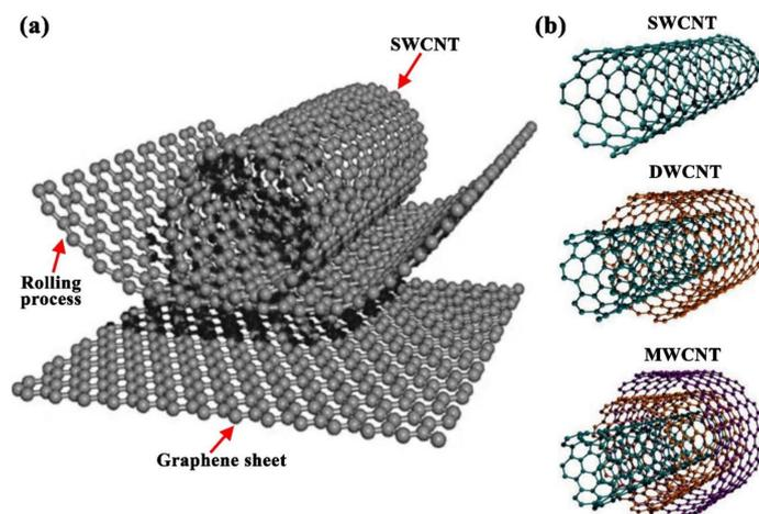
**Figure 3.** Carbon nanotubes formation and classifications, where (a) illustrates the rolling mechanism of graphene sheet into SWCNT and (b) demonstrates the three different categories of CNTs, namely SWCNT, DWCNT, and MWCNT.
