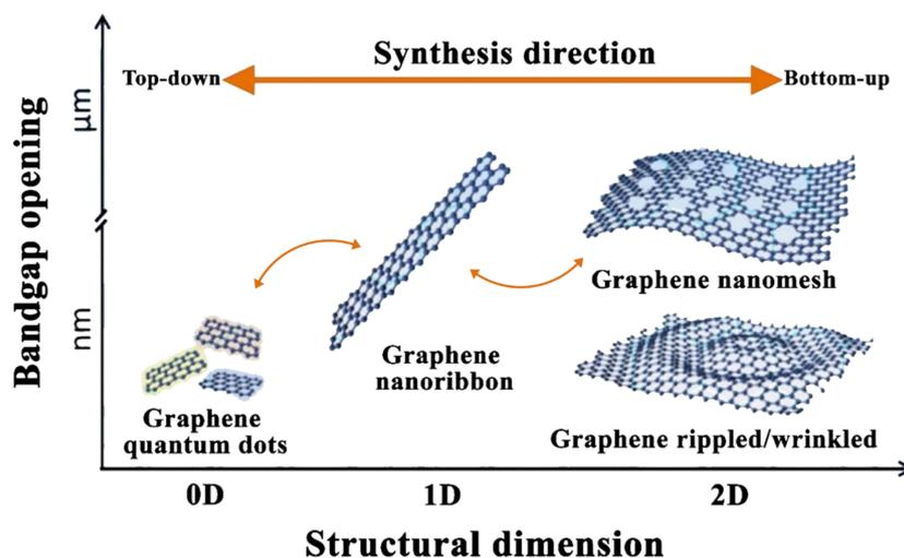
**Figure 2.** Different forms of graphene based on their dimensionality and bandgap opening, where graphene quantum dots, graphene nanoribbon, and both graphene nanomesh and graphene rippled/wrinkled have a structural dimension of 0D, 1D, and 2D, respectively.
