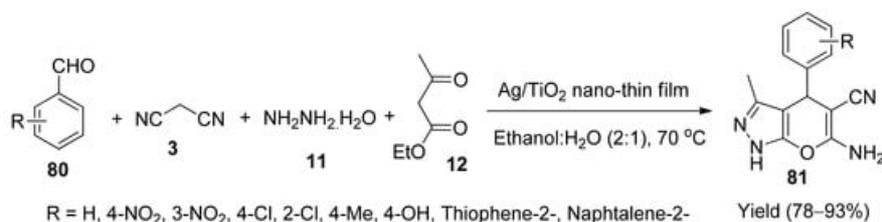
**Scheme 22.** Synthesis of pyranopyrazole derivatives **81** using Ag/TiO<sub>2</sub>.
