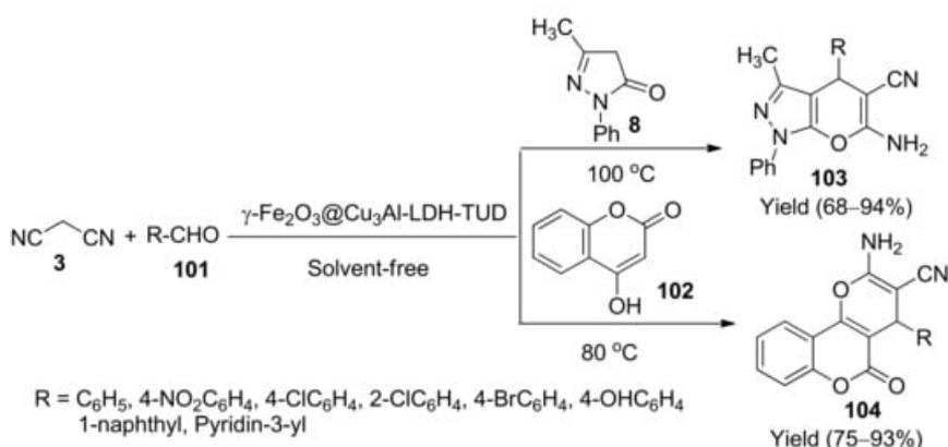
**Scheme 31.** Synthesis of pyranopyrazoles **103** and pyrano[3,2-c]chromenes **104** using  $\gamma$ -Fe<sub>2</sub>O<sub>3</sub>@Cu<sub>3</sub>Al.
