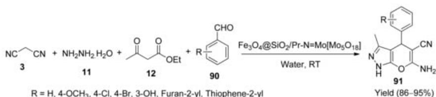
**Scheme 27.** Synthesis of pyranopyrazole derivatives **91** using  $\text{Fe}_3\text{O}_4@\text{SiO}_2$ .
