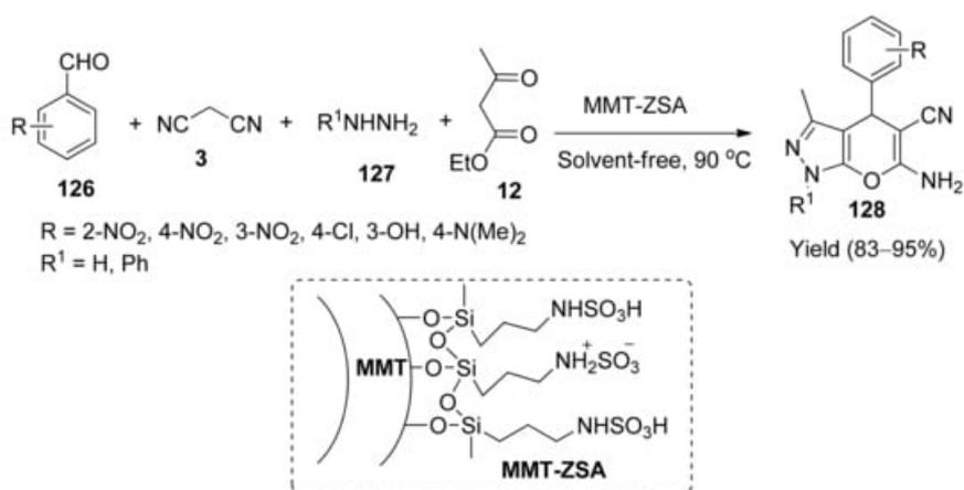
**Scheme 36.** Synthesis of pyranopyrazole derivatives **128** using zwitter-ionic sulfamic acid catalyst.
