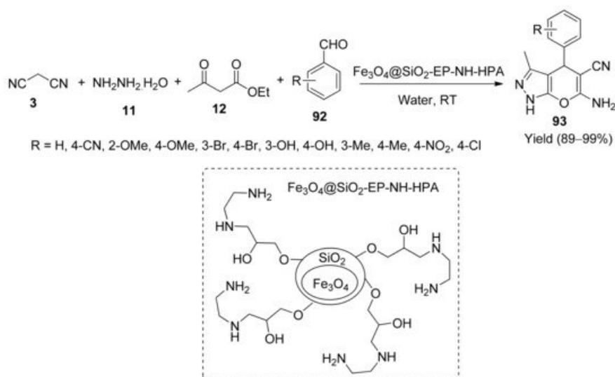
**Scheme 28.** Synthesis of pyranopyrazole derivatives **93** using Fe<sub>3</sub>O<sub>4</sub>@SiO<sub>2</sub>.
