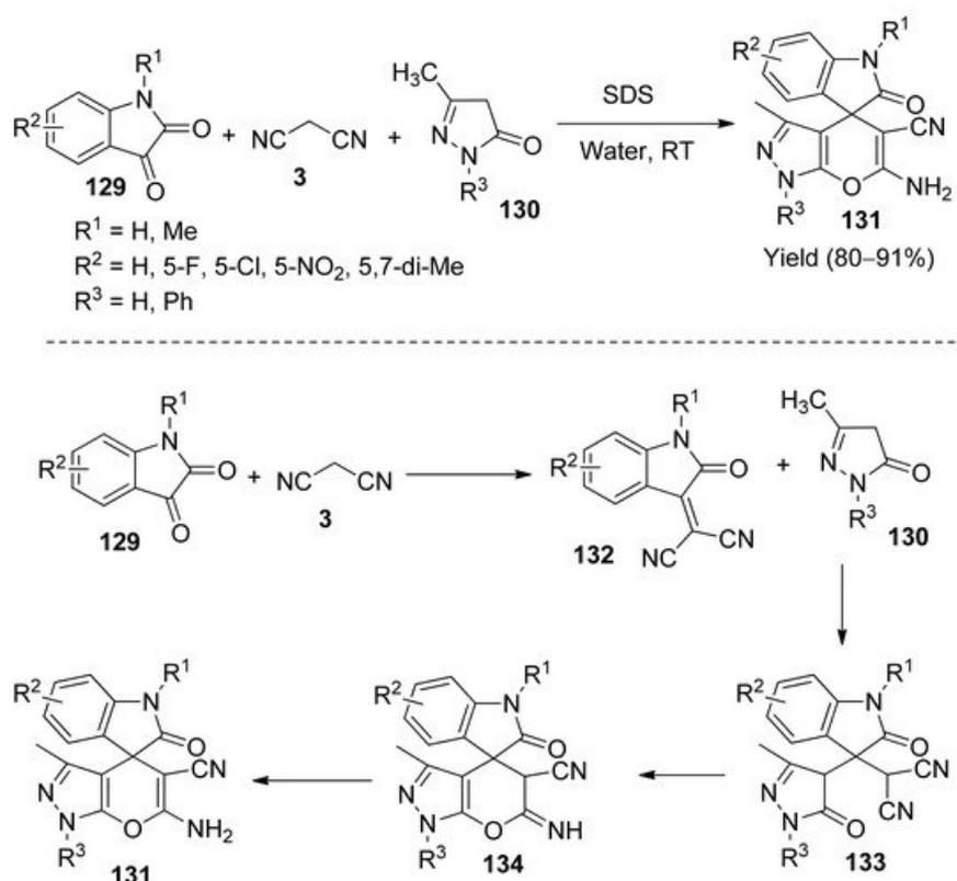
**Scheme 37.** Synthesis of spiro[indoline-pyranopyrazole] derivatives **131** using sodium dodecyl sulfate.
