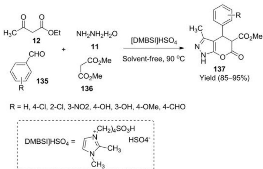
**Scheme 38.** Synthesis of pyranopyrazole derivatives **137** using [DMBSI]HSO<sub>4</sub>.
