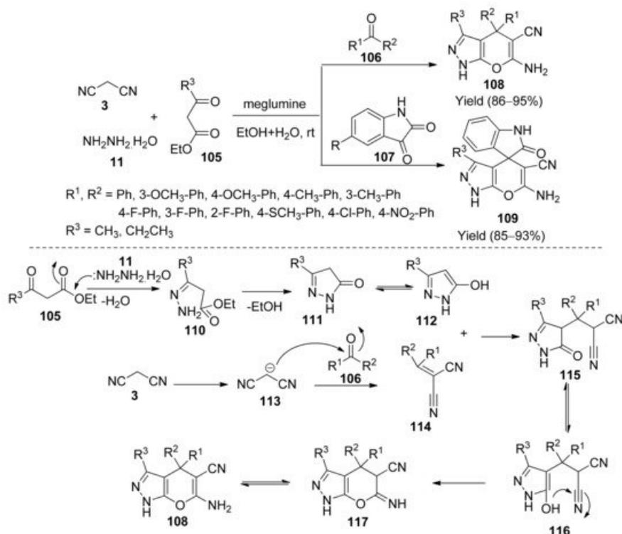
**Scheme 32.** Synthesis of pyranopyrazoles **108** and spiro-pyranopyrazoles **109** using meglumine.
