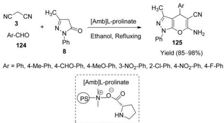
**Scheme 35.** Synthesis of pyranopyrazole derivatives **125** using [Amb]L-prolinate.
