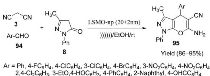
**Scheme 29.** Synthesis of pyrano[2,3-c]pyrazole derivatives **95** using LaSrMnO<sub>3</sub>.
