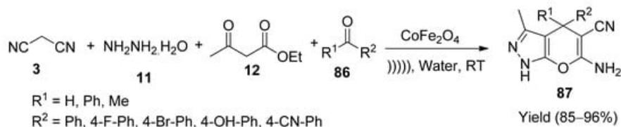
**Scheme 25.** Synthesis of pyranopyrazole derivatives **87** using  $\text{CoFe}_2\text{O}_4$ .
