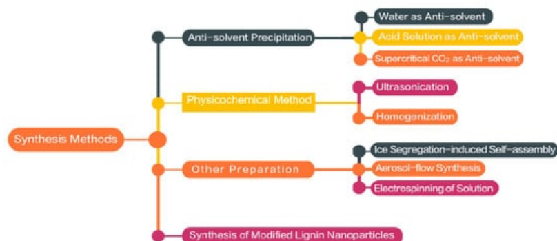
Figure 3. Overview of the synthesis and modification methods of nano-lignin.
