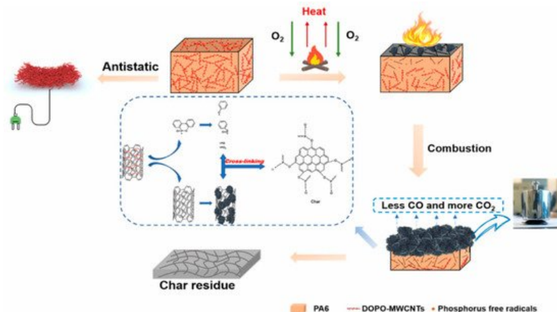
Figure 9. Possible flame retardant and antistatic mechanism of PA6/DOPO multi-walled carbon nanotubes (MWCNTs) [48].
