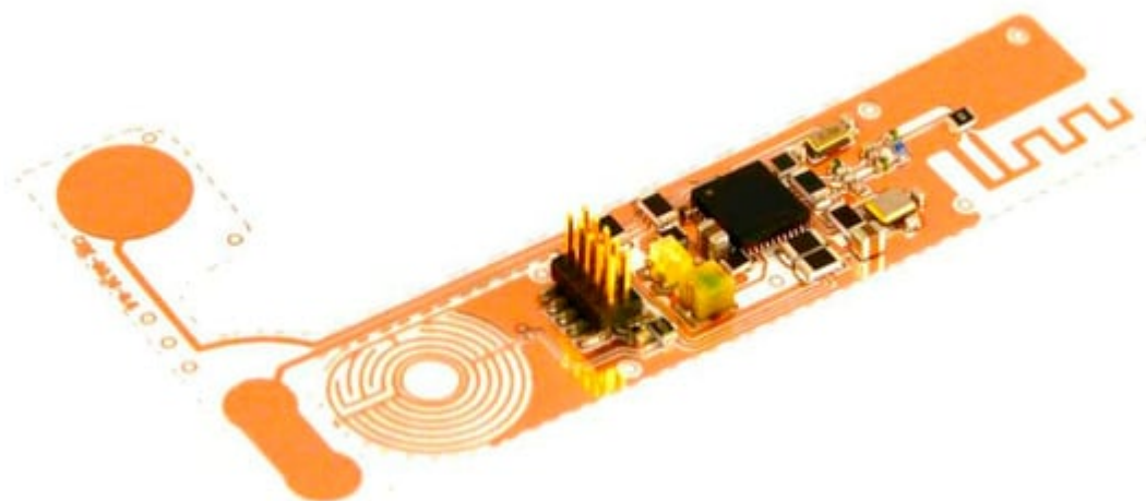
Figure 2. Bluetooth sensor circuit mounted on a flexible substrate. Source: https://www.edn.com/product-how-to-build-your-own-designs-on-flexible-circuit-boards (accessed on 20 March 2021).
