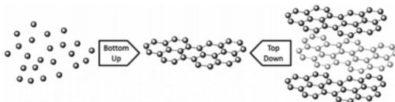
Figure 4. Top-down model and bottom-up synthesis of graphene. “Reproduced with permission from [19] , [Materialia]; published by Elsevier, 2020”.
