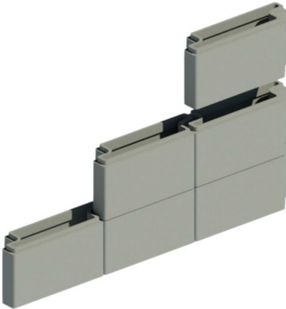
Figure 1. Innovative building envelope designed for 3D printing.
