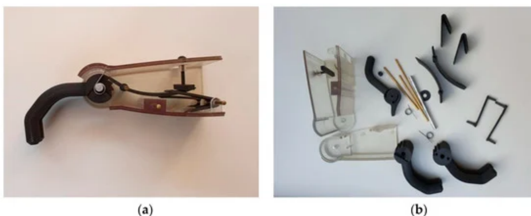
Figure 4. Third 3D-printed polymer replica of the first “Iron Hand” of Götz von Berlichingen with an opening mechanism by a torsion spring. (a) In this photograph, the first finger block, the new thumb lever mechanism, and
