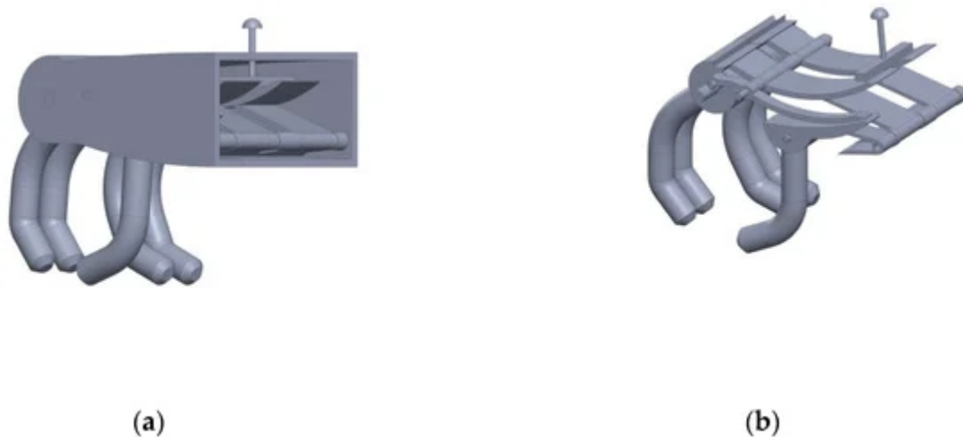
Figure 1. Initial 3D computer-aided design (CAD) reconstruction of the first “Iron Hand” of Götz von Berlichingen. (a) General view of the artificial prosthetic hand; (b) view after virtual removal of the chassis with insight into the mechanics.
