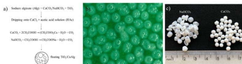
Figure 4. (a) Scheme from ionotropic gelation and CO 2 generation from both gas forming agents (CaCO 3 and NaHCO 3 ), (b) bubbles held within the gel beads with CaCO 3 in its formulation, and (c) floating TiO 2 /CaAlg beads with 1:1 ratio of NaHCO 3 /alginate and 1:1 ratio of CaCO 3 /alginate [24].
