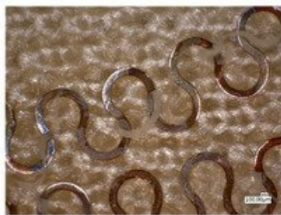
(a) Delamination of protective layer along conductive tracks. (Reprinted from [42])
