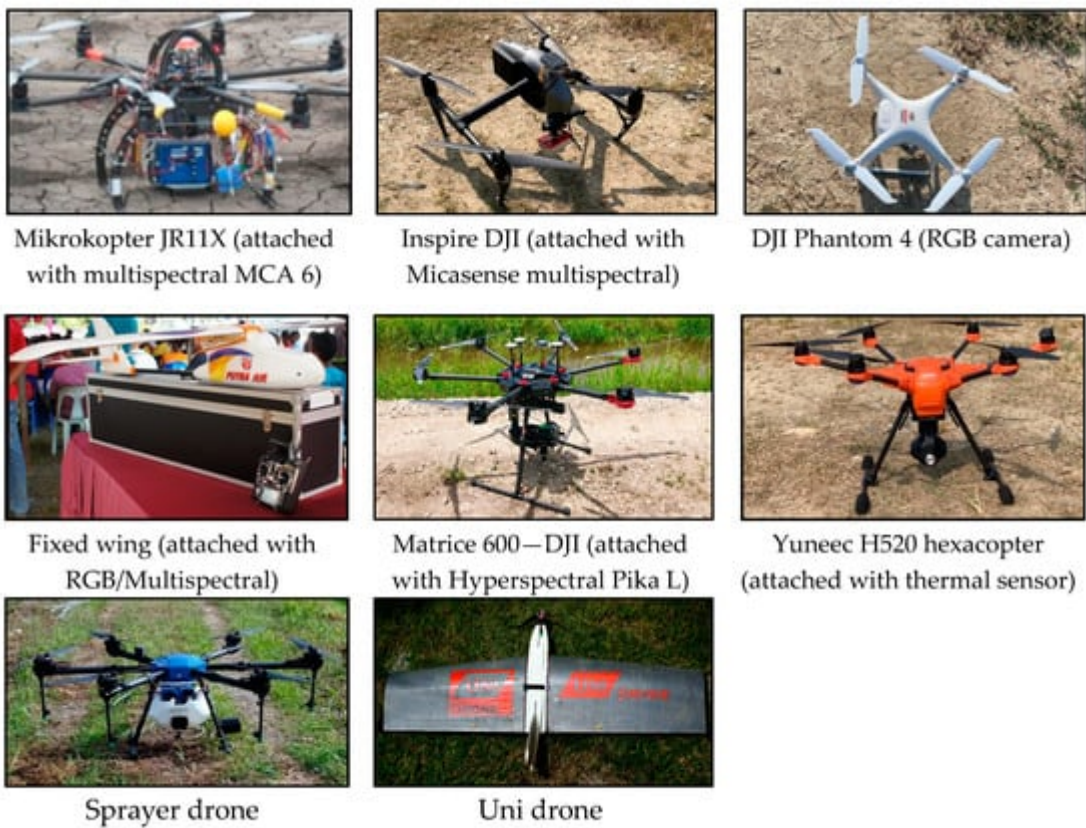
Figure 2. Example of UAV systems used in detecting weed (The pictures were captured by authors).
