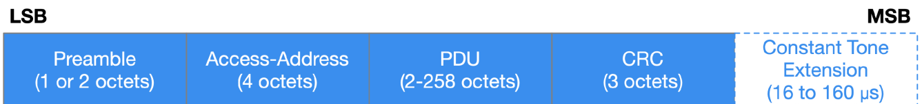
Figure 3. Structure of a Bluetooth 5.1 packet with the duration and position of the CTE. Associated apps add CTE to conventional packets, while those without a connection use an advertizing packet.
