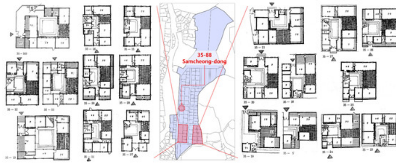
Figure 2. Floor plans of twenty urban-type hanok buildings in 35 Samcheong-dong, near the Samcheong Hanok (Reprinted with permission from ref. [2]. Copyright 1987 Sun-jae Kim).
