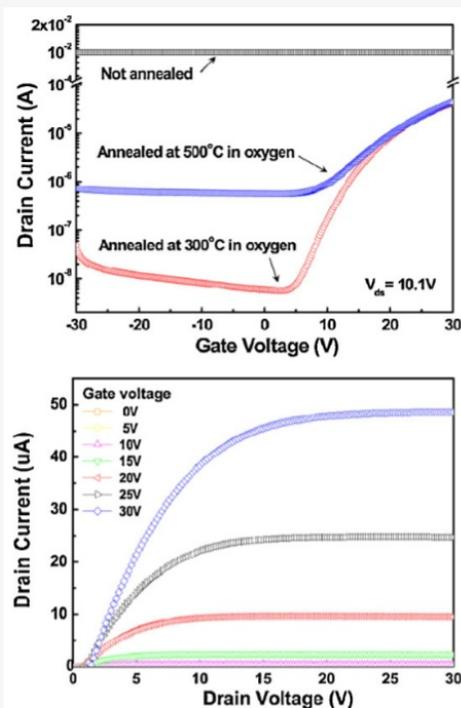
**Figure 2** (online colour at: [www.pss-a.com](http://www.pss-a.com)) Transfer curve of IZO TFT deposited in pure Ar according to annealing temperature (top image) and output curve of the IZO TFT deposited in pure Ar and annealing at 300 °C (bottom image).
