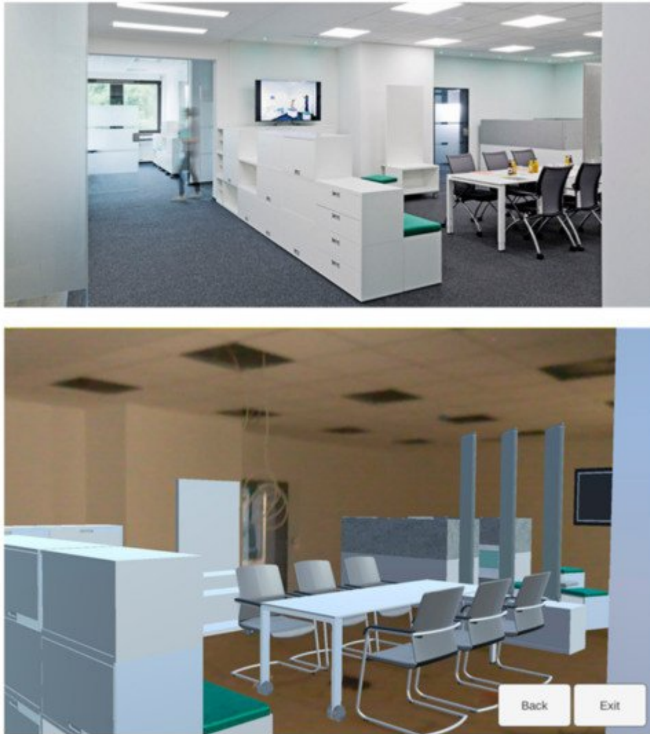
Figure 5. Location of user study: renovated office area with available building information modeling data regarding the building itself as well as the furniture. Top , real furniture after the renovation; bottom , augmented reality visualization during construction [22].
