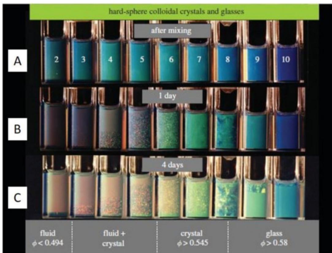
Figure 1. Hard-sphere latex suspensions in cuvettes, illuminated obliquely from behind by white light, (A) immediately after mixing, (B) after 1 day, and (C) after 4 days. In the lowest column (after 4 days), the lower part of the right cuvettes shows the glassy phase with the volume fraction larger than 0.58, the middle cuvettes show the nucleated crystal phase with the volume fraction between 0.545 and 0.58 while the left cuvettes show mostly the fluid phase when the volume fraction is lower than 0.494. Reproduced with permission from [18], Copyright the Royal Society, 2009.
