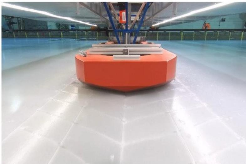
**Figure 6.** A model ship towed through presawn ice at the Aalto ice tank (photo taken by the first author).
