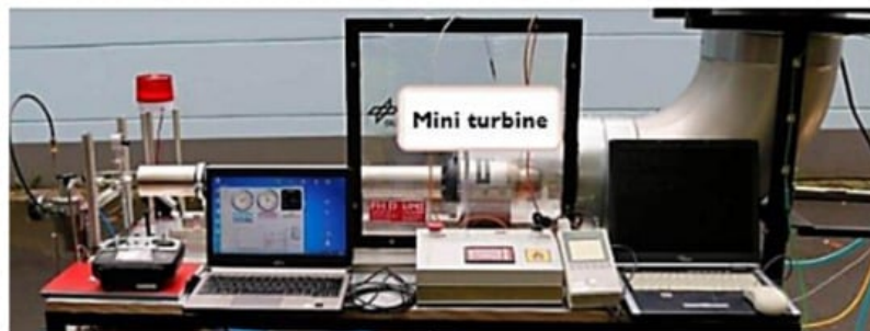
Figure 11. Mini turbine unit used by Naraparaju et al. in their study. Adapted with permission from ref. [82]. Copyright 2018 Elsevier.
