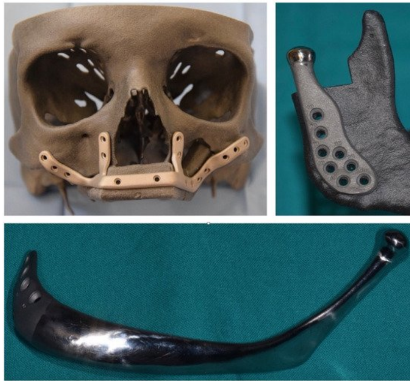
Figure 2. 3D printed implants manufactured by using SLM and used for surgeries at our institution include customized reconstruction plates, temporomandibular joint prostheses, and full mandibular prostheses used for reconstructive purposes in oncologic patients.
