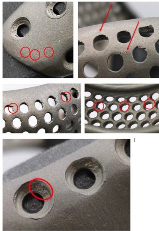
Figure 3. Example of accurate visual inspection conducted on a mandibular prosthesis ordered before MDR entered into force according to the explanations provided in Section 2.2.2 . The manufacturer did not comply with requirements of the new MDR. In particular, undesired amounts of material can be seen on the edges of screw holes, appearing as plugs, clots, or thin leaves. Such imperfections are at risk of detachment during screw fixation and are freed into the body. Moreover, the whole implant surface is filled with small burrs, which are the ideal support for biofilm adhesion.
