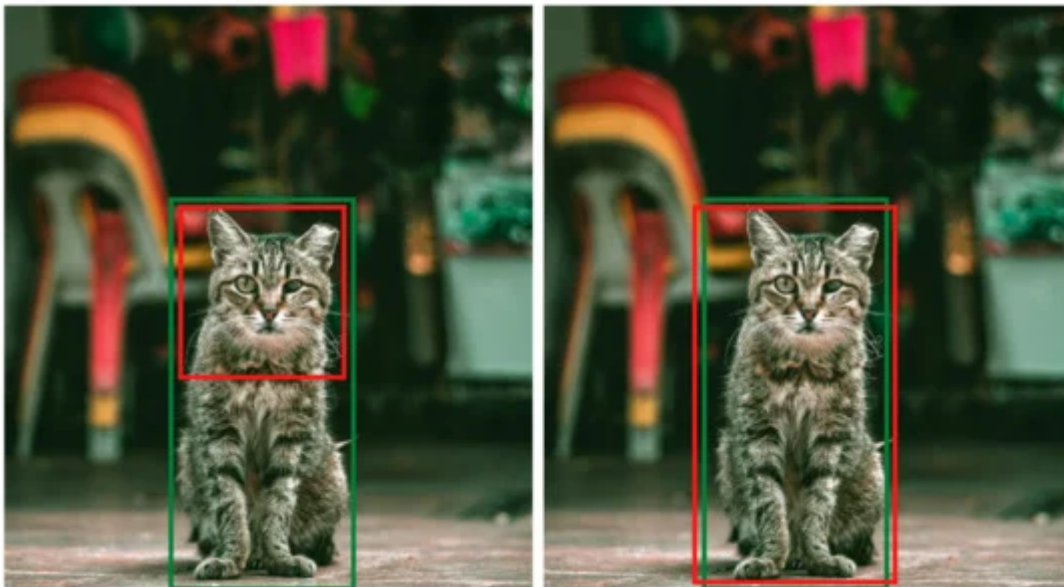
Figure 1. The image explains the visual difference between precise and imprecise prediction in object detection. The green color represents the ground truth, and the red color depicts the predicted boundary. Considering the IOU threshold value equals 0.5, the left prediction is not precise because the IOU between the ground truth and the inferred bounding box is less than 0.5. The bounding box prediction on the right side is precise because it covers almost the complete ground truth area.
