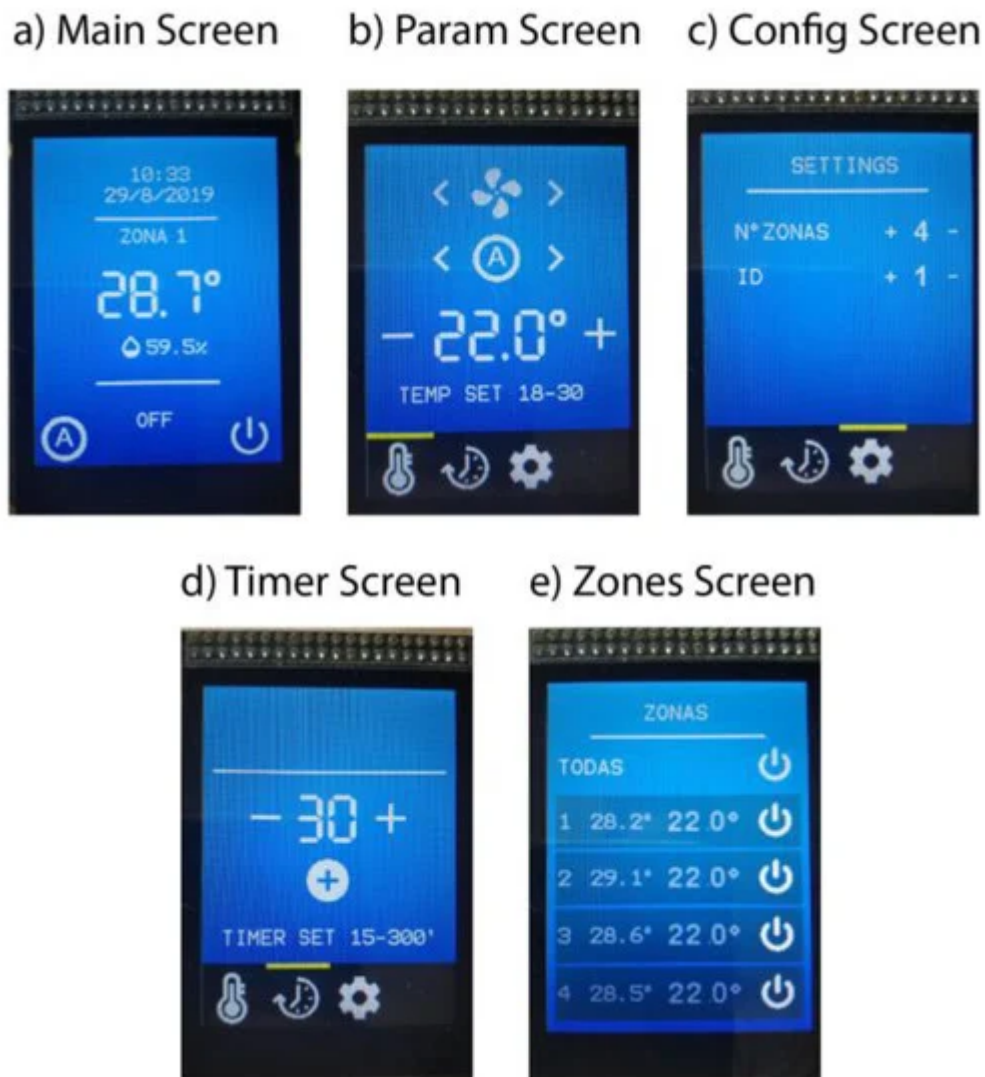
Figure 5. Screens designed for the user interaction: (a) Main screen, (b) Param screen, (c) Config screen, (d) Timer screen, and (e) Zones screen.
