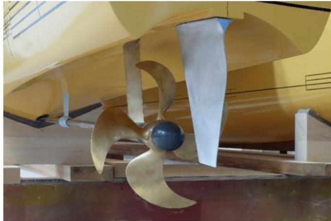
**Figure 3.** Close-up of the transom stern area of the tested Stavanger model, with fitted propellers, shafts, brackets and rudders [\[17\]](#).
