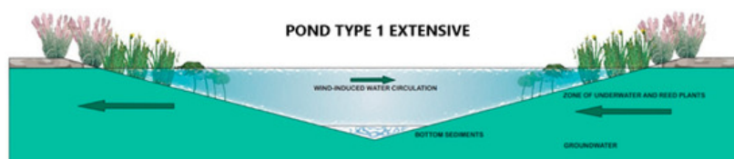
Figure 3. Diagram of the operation of an extensive swimming pond (type 1).
