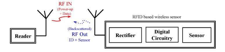
An antenna is a transducer that converts free space electromagnetic energy to guided electromagnetic energy and vice versa to enable wireless communication in an RFID system. Although any radiating structure can be termed as an antenna, the efficiency with which it can transform the electromagnetic energy plays a major role in determining its amenability for use in sensor communication [23].
