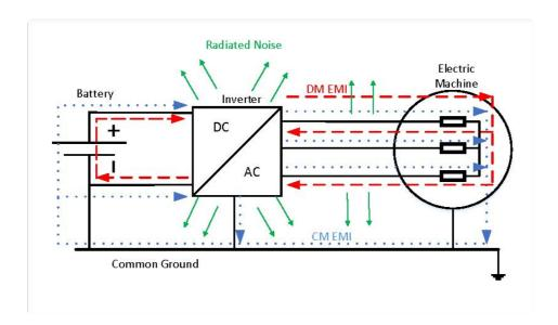
The dashed line represents the differential-mode EMI, which is going through one phase and returns across the other phases to the DC bus of the power source. Finally, the dotted line is the common-mode EMI, which goes
