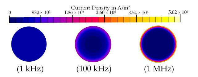
This surface distribution of the current increases the resistance and decreases the inductance due to the flux distribution inside the conductor. The skin effect is a local effect in each conductor, independent from the neighboring ones, so it can be analyzed simplifying the problem to a single conductor [23][24]. As it depends on the frequency and geometry, it can be mitigated using a smaller conductor diameter than the skin depth.
