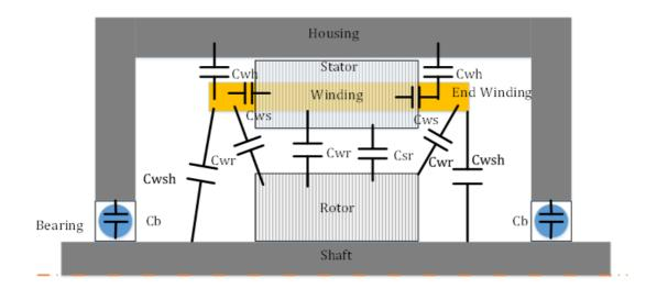
In the winding, different capacitances appear. The inter-turn capacitance and the capacitance between phases that can be neglected if there is a single layer winding in the slot [27]. The complete common-mode (CM) paths are identified in [14]. To calculate the inter-turn capacitances, it is essential to consider the geometry, material and positions of the conductors inside the slot, as well as the thickness and the material of the insulation [32][33].
