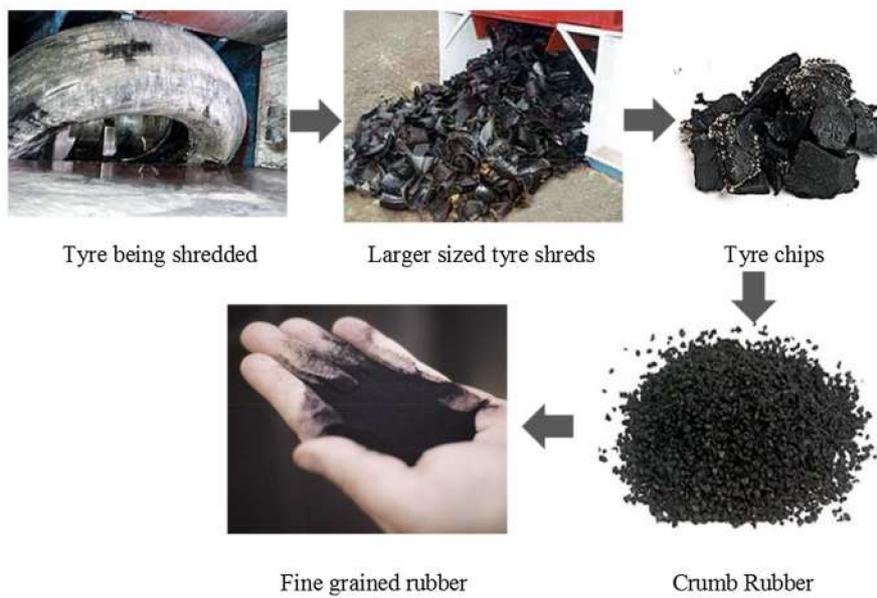
**Figure 3.** Different stages of tire shredding [4].
