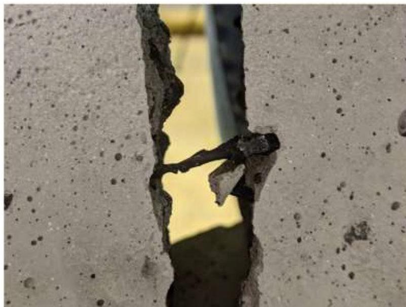
**Figure 4.** Crack bridging by tire shreds [5].
