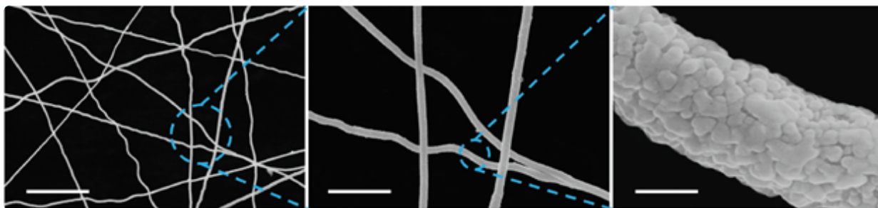
Figure 3. SEM image of AgNW network (scale bar 10 and 2 \mu\text{m} and 300 nm) [27].
