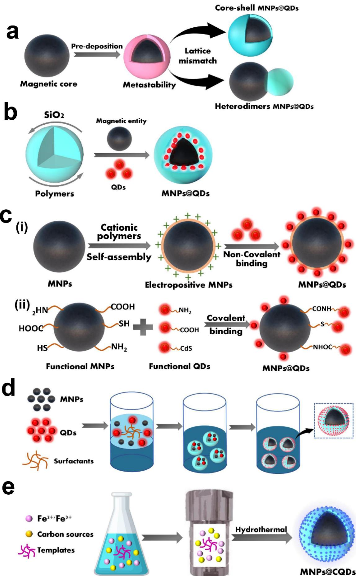
**Figure 1.** Schematic diagram of five preparation methods of MNPs@QDs nanocomposites. (a) Hetero-crystalline growth; (b) Template embedding; (c) Layer-by-layer assembly constitute of (i) non-covalent binding and (ii) covalent binding; (d) Microemulsion technique; (e) One-pot method.
